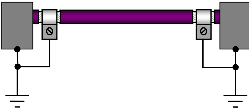
Figure 3-32 Standard grounding concept for PROFIBUS
